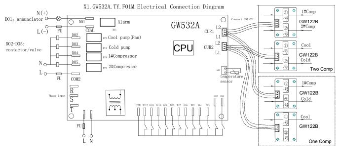
DI1:Cool overload/Antifreezing switch DI2:Remote switch DI3:Cold Pump overload DI4:Cold Water flow switch DI5:Water level switch/Vent1 temperature DI6:1#Compressor overload DI7:Low pressure of 1#compressor DI8:High pressure of 1#compressor DI9:Cool flow switch/Vent2 temprature/Phase switch DI10:2#Compressor overload DI11:Low pressure of 2#compressor
